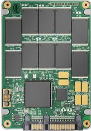
Inside the SSD: no moving parts.
